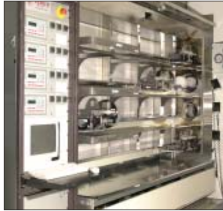
Semco 4 Tube Furnace Stack
